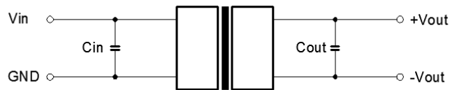
Figure 1: Typical External circuit
